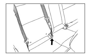
Flip the bottom seat cushion forward by pulling up on the tab located in the center of the seat cushion where the seatback meets the seat cushion. There is a tab on both rear seats.
